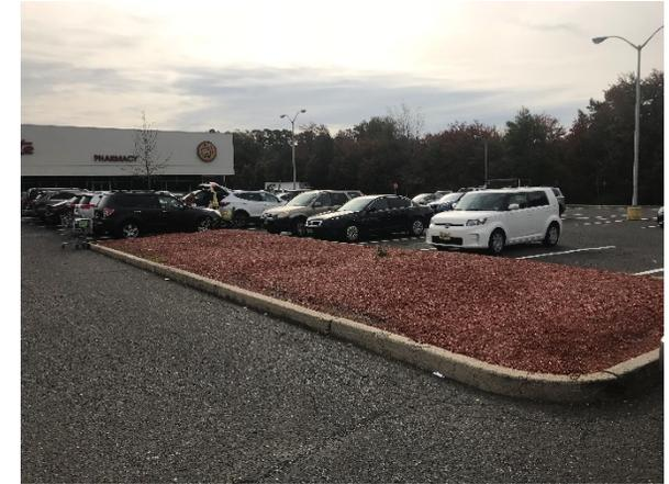
Sections of parking spaces can be converted to porous pavement to capture and infiltrate stormwater runoff from the parking lot. A parking lot island can be converted to a rain garden to capture, treat, and infiltrate stormwater runoff from the parking lot as well. A preliminary soil assessment suggests that the soils have suitable drainage characteristics for green infrastructure.
