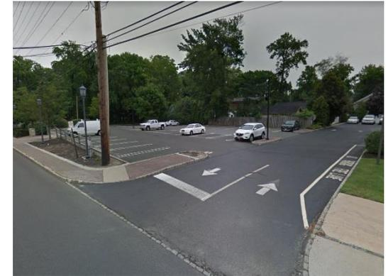
A section of parking spaces can be converted to porous pavement to capture and infiltrate stormwater runoff from the parking lot. A preliminary soil assessment suggests that the soils have suitable drainage characteristics for green infrastructure.
