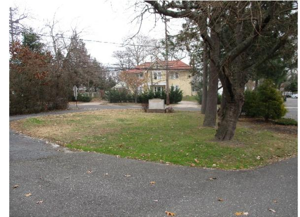
A rain garden can be installed in the turfgrass area in the front of the main building of the golf course to capture, treat, and infiltrate stormwater runoff from the road. A preliminary soil assessment suggests that the soils have suitable drainage characteristics for green infrastructure.
